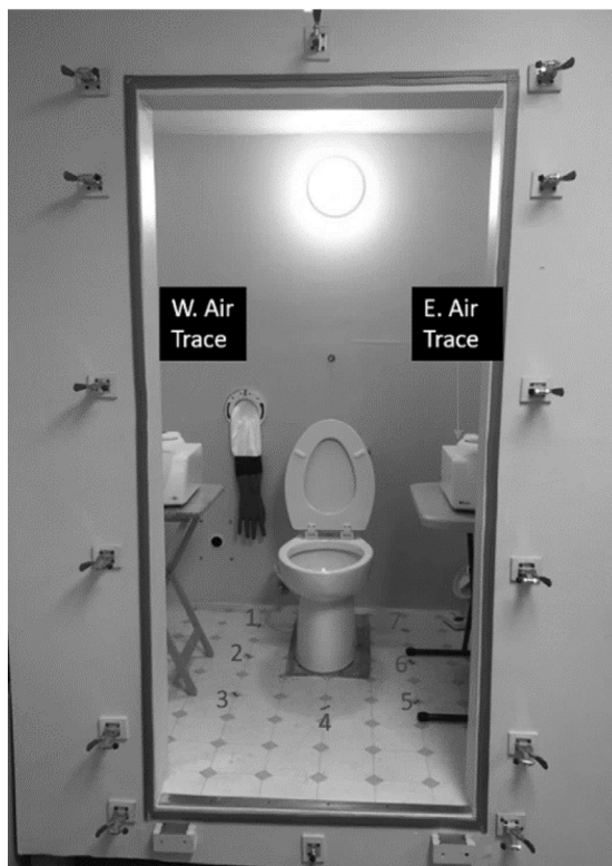
Fig 1. Water closet chamber showing the placement of slit-to-agar bioaerosol samplers, East (E.) and West (W.), and the marked floor locations where surface collection took place.
